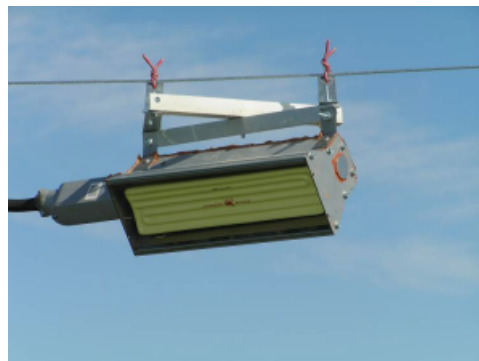
Fig. 1 'Mor FTE' infrared heater deployed at an angle of 45° from horizontal and of 30° with respect to the suspension cable.
